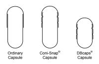
**Figure 3.2** Drawings of an ordinary capsule (left), a Coni-Snap<sup>®</sup> capsule (center) and a DBcaps<sup>®</sup> capsule (right). In Coni-Snap<sup>®</sup> and DBcaps<sup>®</sup> capsules, the tapered rim of the body is designed to avoid telescoping, the grooves on cap and body lock together; the presence of indentations prevents premature opening.
