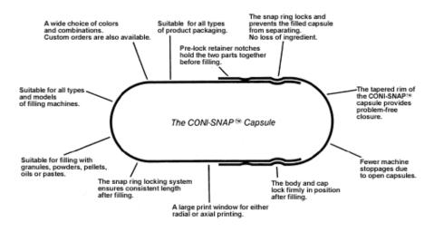
**Figure 3.1** Chart indicating the characteristics of the Coni-Snap<sup>®</sup> capsule (Capsugel: Pfizer, Inc.).
