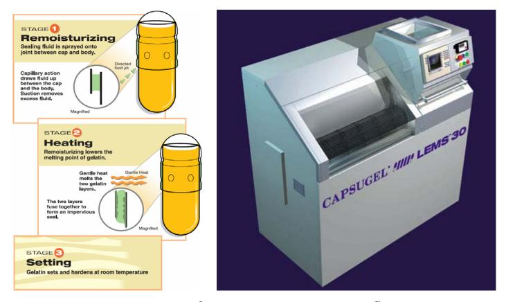
**Figure 3.5** (Left) Sealing mechanism for Licaps<sup>®</sup> capsules and (right) the Capsugel LEMS<sup>™</sup>30 (Liquid Encapsulated Microspray Sealing) capsule-sealing equipment (Capsugel: Morris Plains, NJ).
