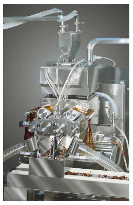
**Figure 3.9** A rotary-die soft gelatin capsule filler (Pharmagel Engineering SPA: Milan, Italy)
